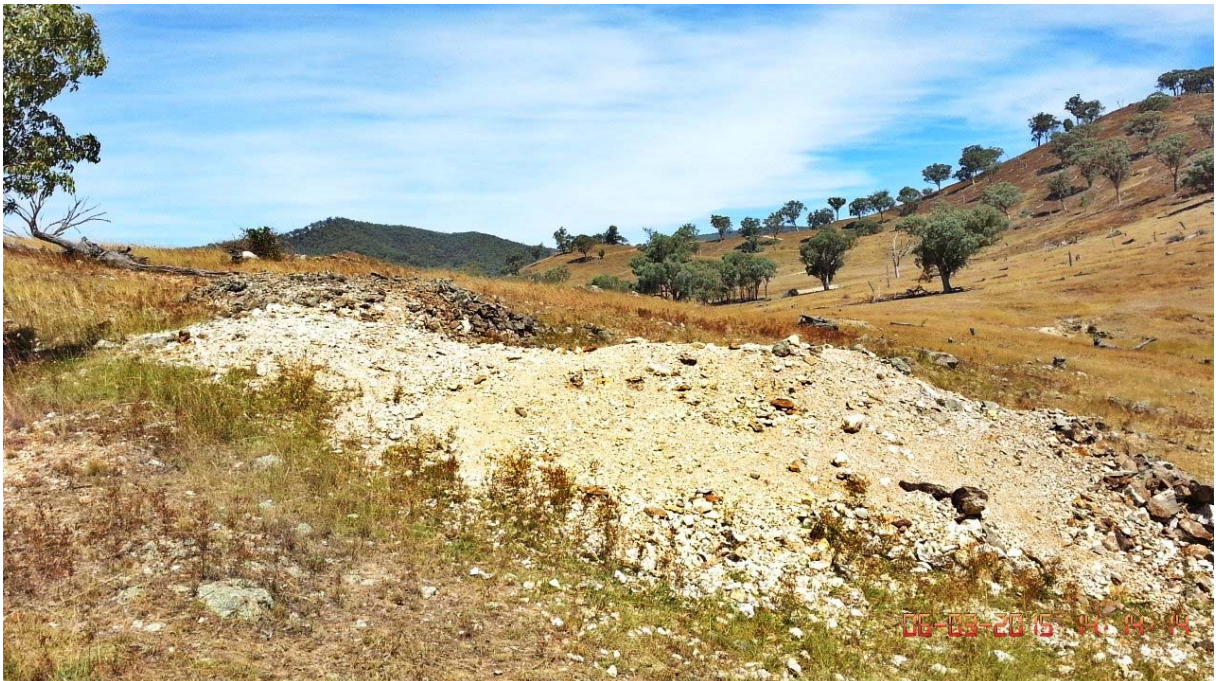
Figure 3. Quartz ore coarse reject stockpile from early mining at Reef Hill (main shaft out of picture to the left). A sample of the quartz returned 1.1 g/t gold.
