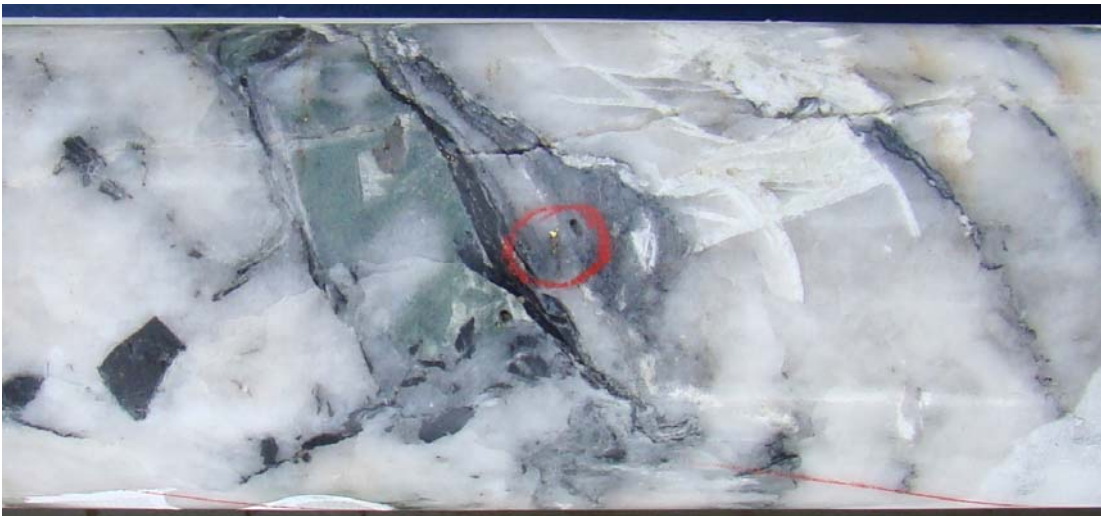
Visible gold in a quartz vein fault breccia from a mineralised interval in the first drill hole of the North Big Nugget Hill drilling program (HGD058 at 70.1m). The photograph is from a mineralised interval of 6.4m.
